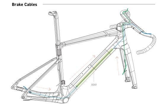
Step 5.4 Rear brake cable: Route the rear brake cable through the left chainstay, running through the bottom bracket and exiting through the top of the head tube. Cut a [OD01] foam cable sleeve to a similar length as the down tube, slide onto the cable, and adjust the sleeve's position to sit inside the down tube.
