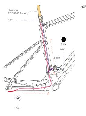
Shimano Di2 shifters are wireless, therefore there is no need to connect shifter cables to the handlebars.
