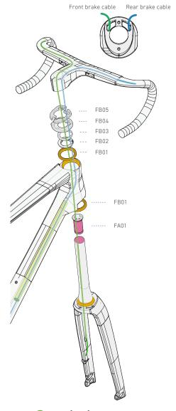
Thin [FB03] 0.2mm headset washers are provided in case more clearance is needed, they can be excluded or included as the situation requires. Step 5.6 In the correct order, thread the [FB01] top headset bearing, [FB02] headset compression ring, [FB04] headset cap, and [FB05] headset spacer onto the steerer tube and brake cables. The brake cables then enter the AER01v stem from its bottom cable holes, and come out through the ends of each handlebar with the help of a cable routing kit.
