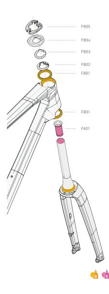
Step 3.1 Prepare the frame, fork, headset bearings, headset cap, headset washers, stem, and handlebar, and confirm the number of headset washers needed below the stem.
