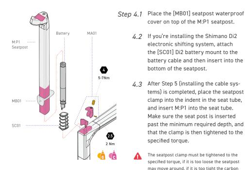
When placing the [MA01] seatpost clamp, tilt the bike 30 ~ 60 degrees or use tape to prevent the clamp from falling into the seat tube.
