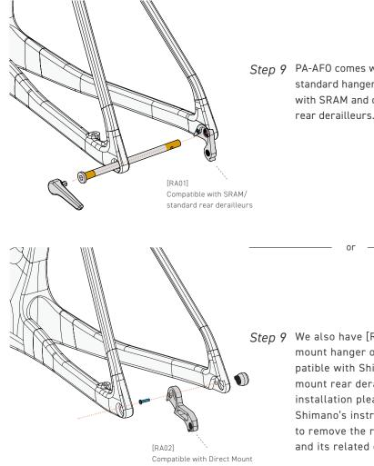
Step 9 PA-AFO comes with a [RA01] standard hanger compatible with SRAM and other standard rear derailleurs.
