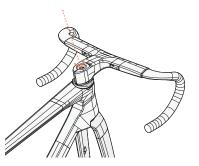
The plug expander must be tightened to the specified torque only after the stem has been installed, in order to avoid over-expansion.
